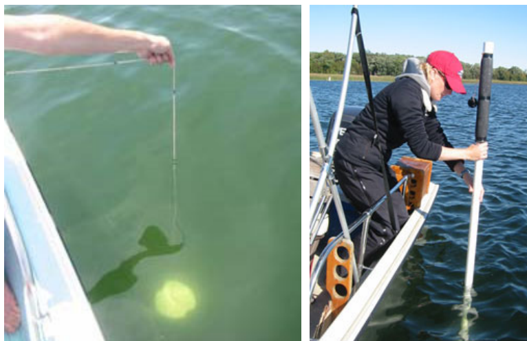
Figure 8-3. Monitoring a lake with a Secchi disk and a 2-meter integrated sampler.
